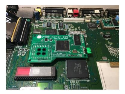
The correctly installed Wicher 608 card is ready for use.
